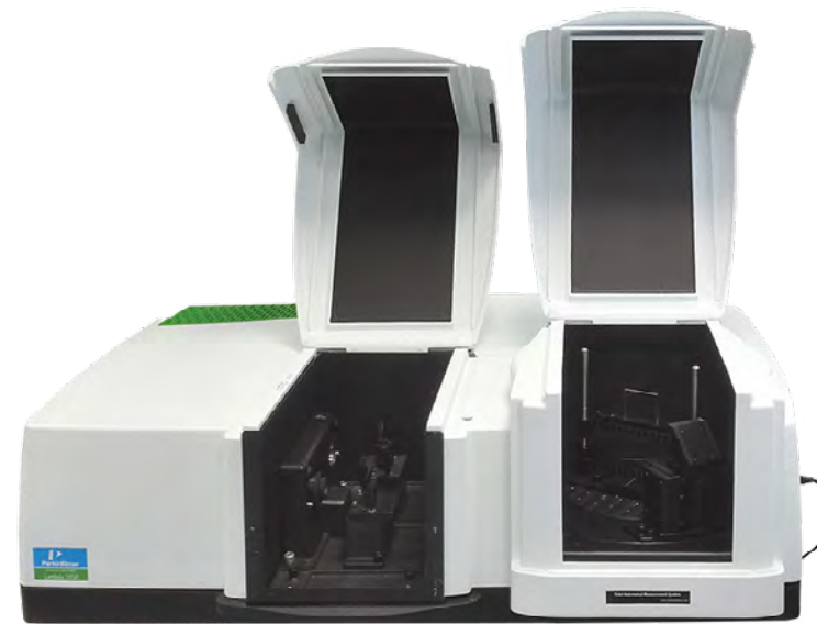
LAMBDA 1050 UV/Vis/NIR Spectrophotometer with Total Absolute Measurement System (TAMS)
