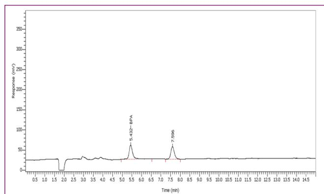
Figure 3: BPA calibration standard at 1 ppb.
